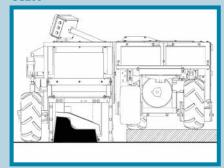
DROP POUR MODE, PAVEMENT TO SUBGRADE ADDITIONAL DROP ADAPTER REQUIRED
